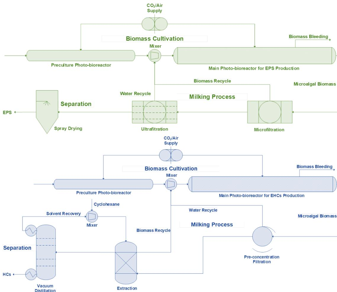
Figure S1. Flowsheets for the production of EPS in S1a/S1b (up) and HCs in S2a/S2b (down).
