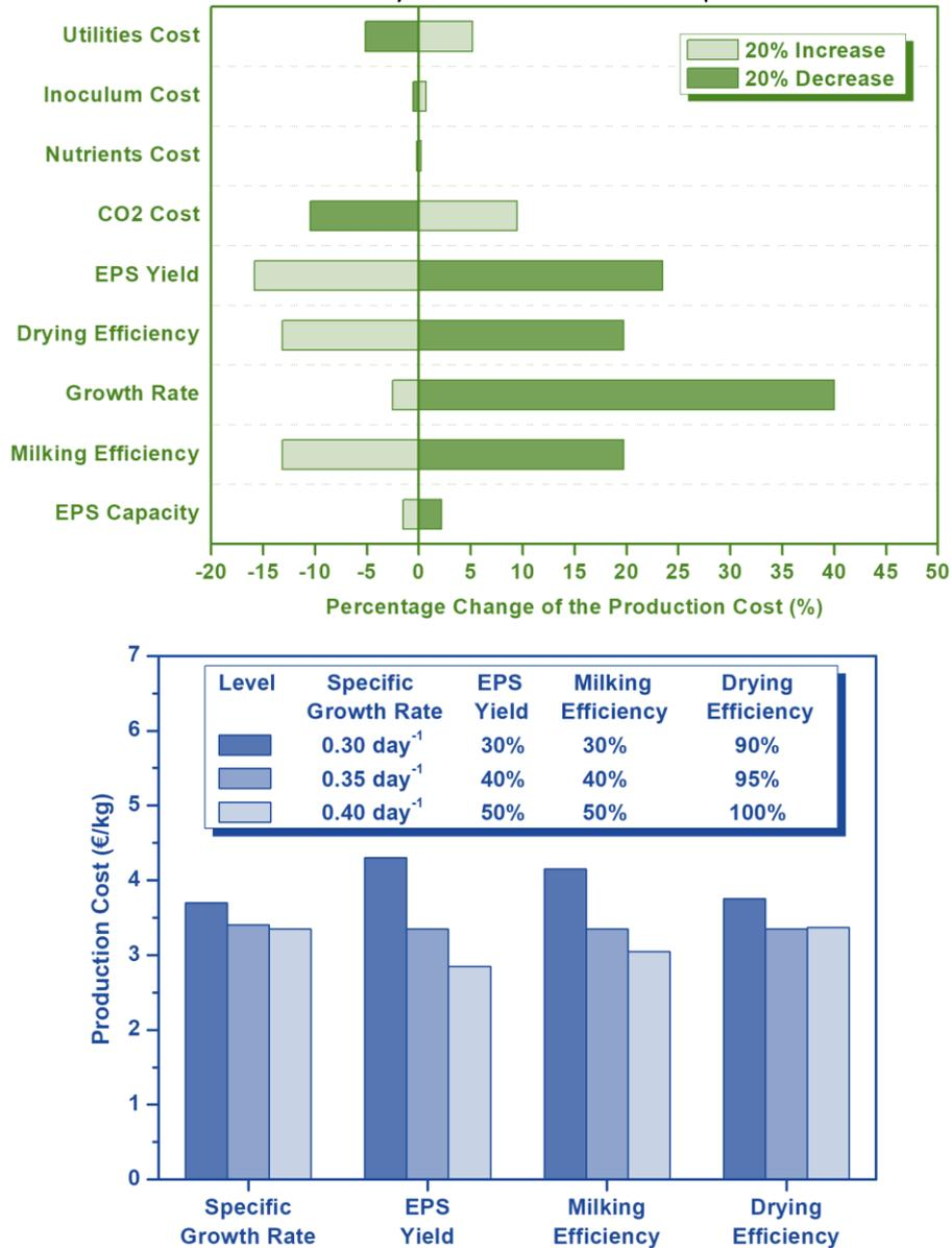
**Figure S2.** First (up) and second (down) level sensitivity analysis of the selected key-process parameters impact on the production cost for scenario S1a.
